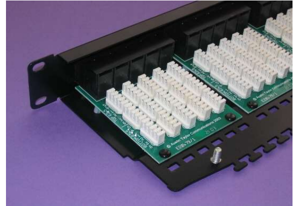
Rear of high-density voice patch panel showing IDC connections, pair labelling and single earthing point per PCB.
