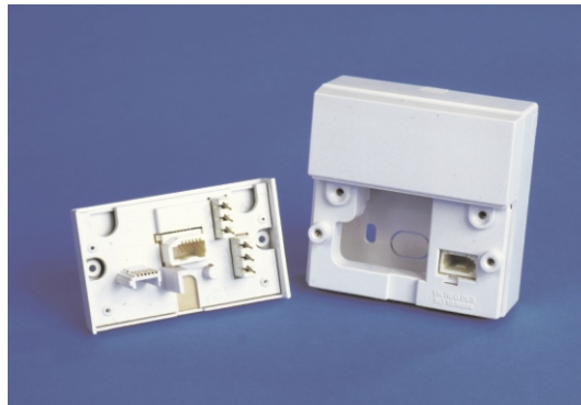
NTE5 with user access cover removed showing test socket in base and connection point for customer extension wiring in cover
